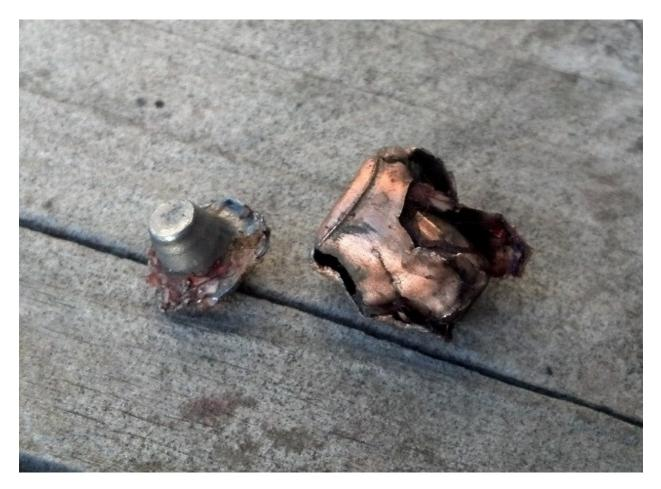
The same bullet with the core removed which fell away easily. If you look closely, you will note that after reaching the Interlock swage in the jacket, the core then gradually continued forwards, shedding weight as it did so. In other words, the core can slip (compare the length of the core shank to the length of the jacket). Nevertheless, the core and jacket were in this instance found together. Other fragments ((85 grains worth) created broad wounding.
