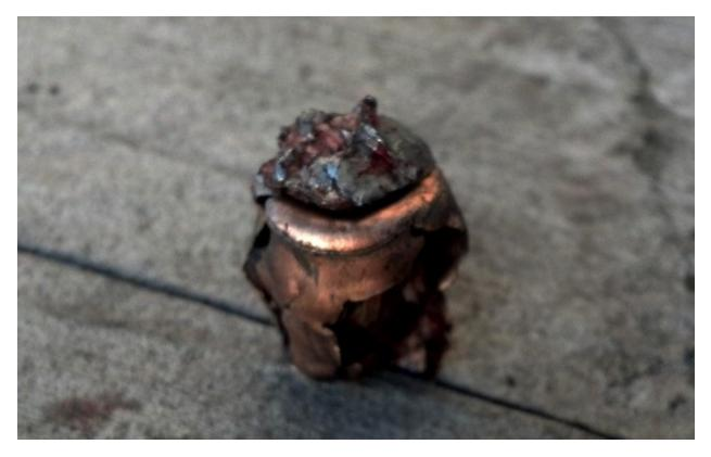
The 200gr ELD-X after a raking shot at an impact velocity of 2300fps. Retained weight 115 grains. Wounding is violent whether tackling light or large bodied animals, penetration is very good considering the nature of this bullet design. Note also how the frontal area has reduced, the jacket folding back into itself rather than a wide frontal area which could arrest the bullet early on.
